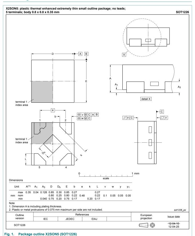
plastic, leadless thermal enhanced extremely thin small outline package; no leads; 5 terminals; 0.48 mm pitch; 0.8 mm x 0.8 mm x 0.35 mm body
